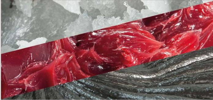
The colors of greases are simply dyes chosen by the manufacturer. They have no standardized meaning. For example, red does not signify high temperature performance, and blue does not mean electric motor bearing grease.
