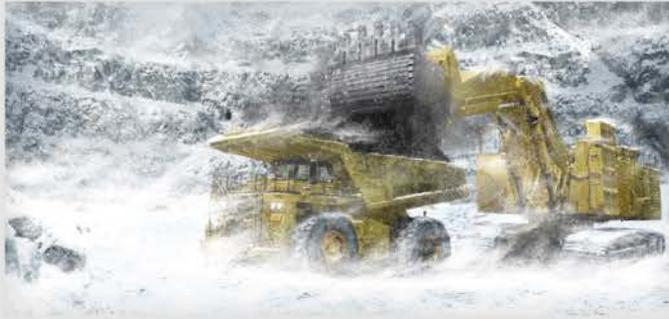
Cold temperature pumpability is a real concern if grease is exposed to cold ambient temperatures. You may need to switch between a thinner grease in the winter (e.g. NLGI #0 or #1) and a harder grease #2 in the summer, or select an appropriate multi-season grease for year-round use.
